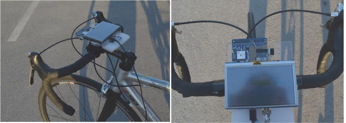
Fig. 3: Deployment of the AST-Monitor on a real cycle.
