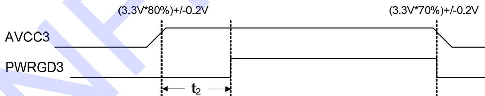
**Figure 11-9. ACPI Power Signal Timings**
