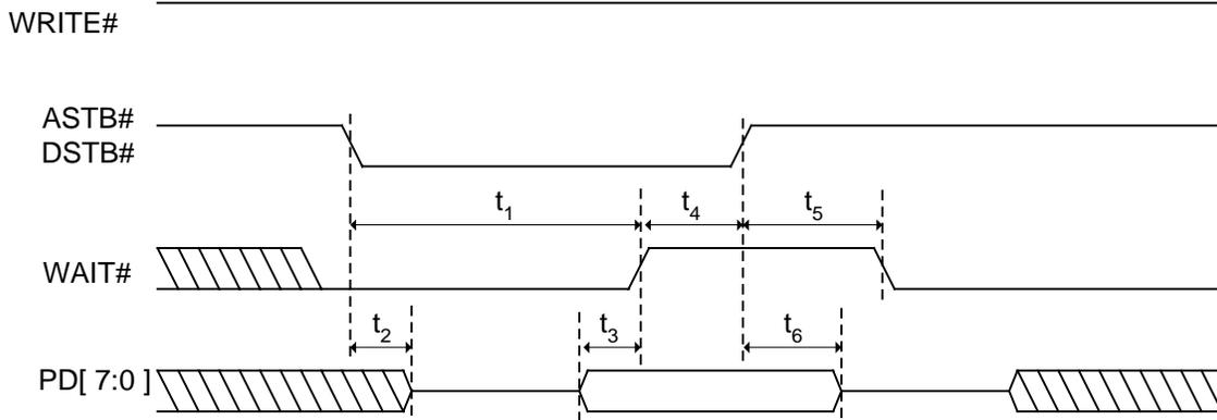
Figure 11-8. EPP Address or Data Read Cycle Timings
