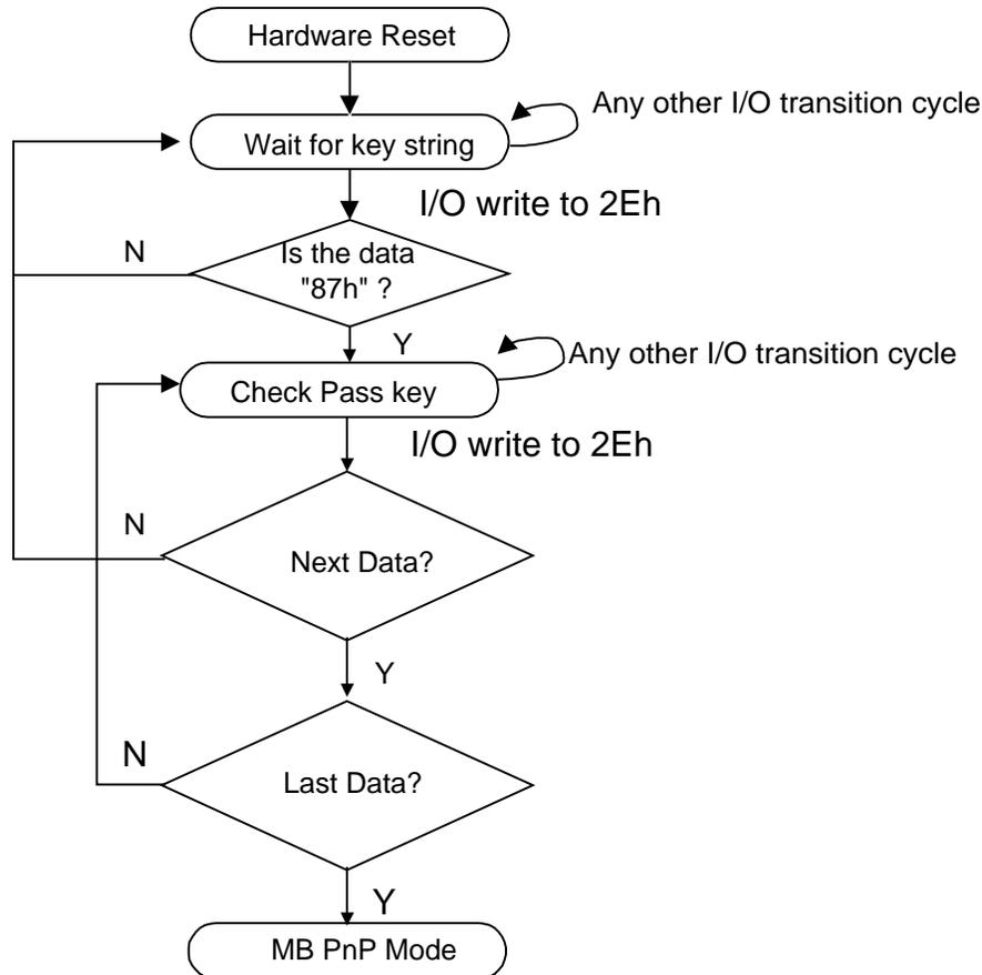
There are three steps to completing the configuration setup: (1) Enter the MB PnP Mode; (2) Modify the data of configuration registers; (3) Exit the MB PnP Mode. Undesired result may occur if the MB PnP Mode is not exited normally.
