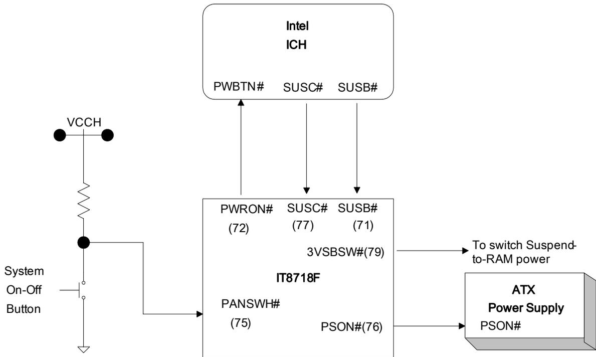
**Figure 7-1. IT8718F Special Applications Circuitry for Intel ICH**
