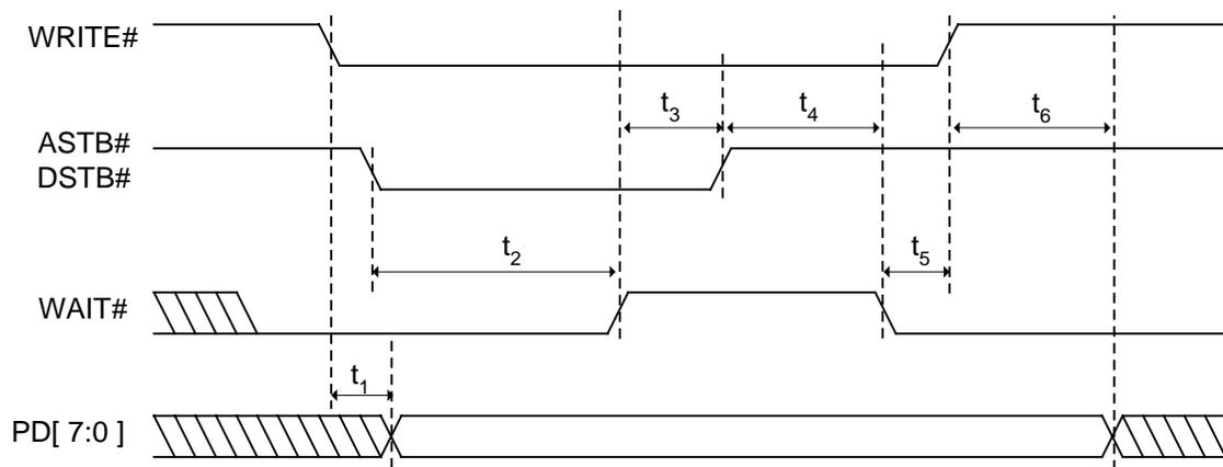
**Figure 11-7. EPP Address or Data Write Cycle Timings**
