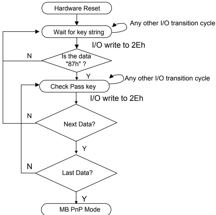
There are three steps to completing the configuration setup: (1) Enter the MB PnP Mode; (2) Modify the data of configuration registers; (3) Exit the MB PnP Mode. The undesired result may occur if the MB PnP Mode is not exited normally.
