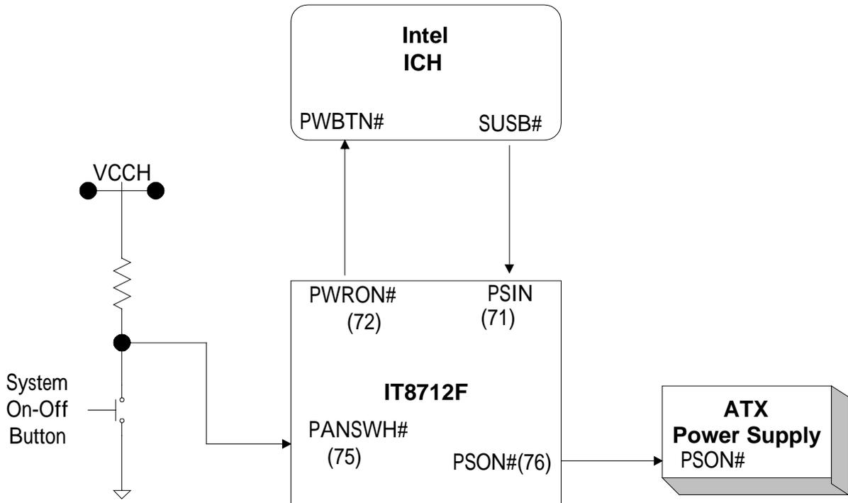
**Figure 7-1. IT8712F Special Applications Circuitry for Intel ICH**
