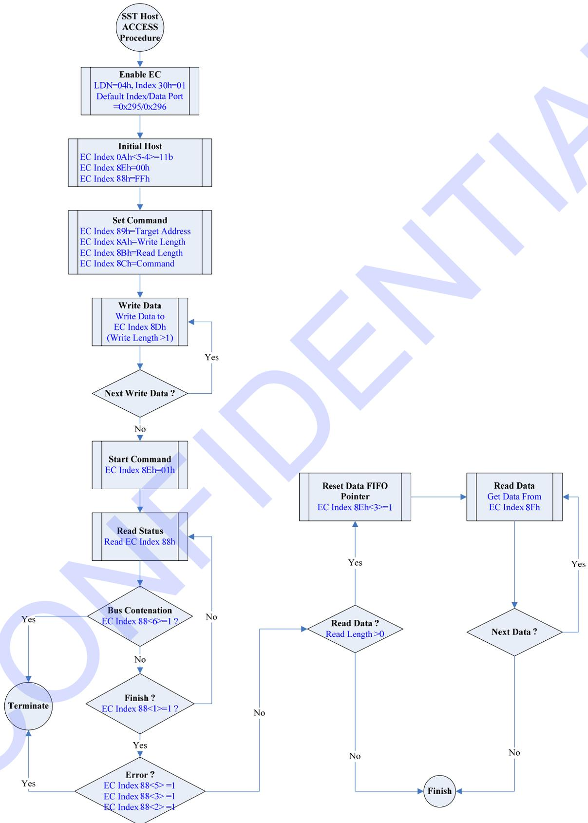
Figure 9-9. SST Slave Programming Procedure
